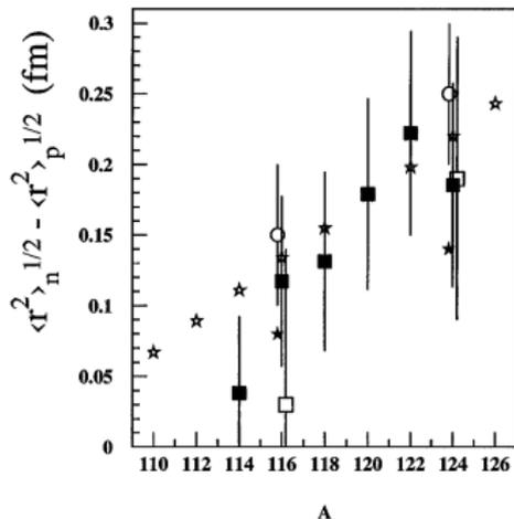
FIG. 3. The difference of the neutron and proton root-mean-square radii as a function of the mass number of the Sn isotopes. The full squares with error bars show the present results. The previous experimental results measured in  $\rho, \rho^0$  reaction [5] and by using the GDR excitations [6] are shown as open circles and squares with error bars, respectively. The open and full stars show the theoretical results of Angeli *et al.* [19] and Dechargé *et al.* [21], respectively.
