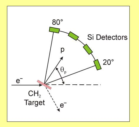
simultaneous measurement of complete angular distribution
