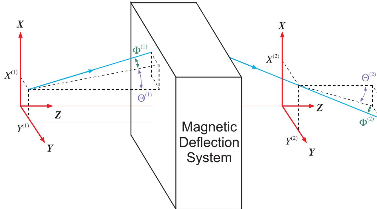
$$\begin{aligned}x_2 = & (x/x)x_1 + (x/\Theta)\Theta_1 + (x/\delta)\delta + \\ & + (x/x_2)x_1^2 + (x/x\Theta)x_1\Theta_1 + (x/\Theta^2)\Theta_1^2 + (x/x\delta)x_1\delta + (x/\Theta\delta)\Theta_1\delta + \\ & + (x/\delta^2)\delta^2 + (x/y^2)y^2 + (x/y\Phi)y_1\Phi_1 + (x/\Phi^2)\Phi_1^2 + \\ & + \text{higher order terms}\end{aligned}$$
