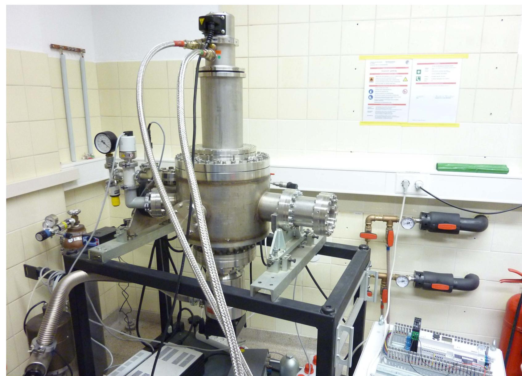
Test chamber for pressure and cooling tests
